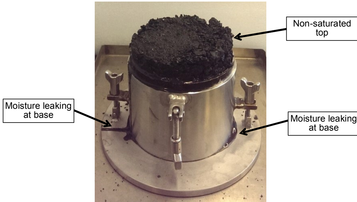
Figure 1.5.8 Test showing water leakage from the base of the cylindrical mould indicating moisture migration
